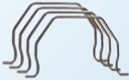
Steel pipe 13 x 1,5 mm, bent on TUBOTRON 20
